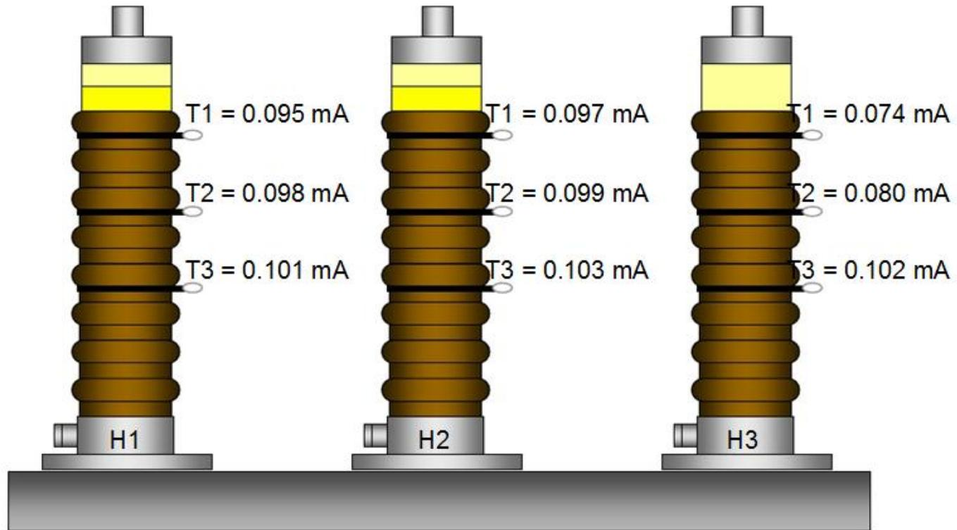
Conclusion: The oil level in the H3 bushing is somewhere between the locations used for tests hot-collar tests 2 and 3.
