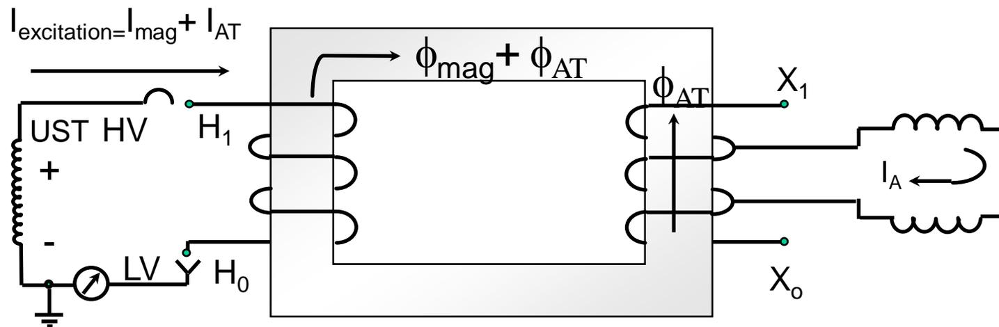
When an autotransformer is connected across two taps it acts as a load and the primary current goes up.
