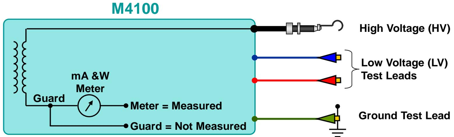
**Kirchoff's Current Law** – All current leaving must return. Therefore, by KCL all current leaving the test set through the HV Cable must return to it ... either through the LV Test Leads (red or blue) or the Ground Lead.
