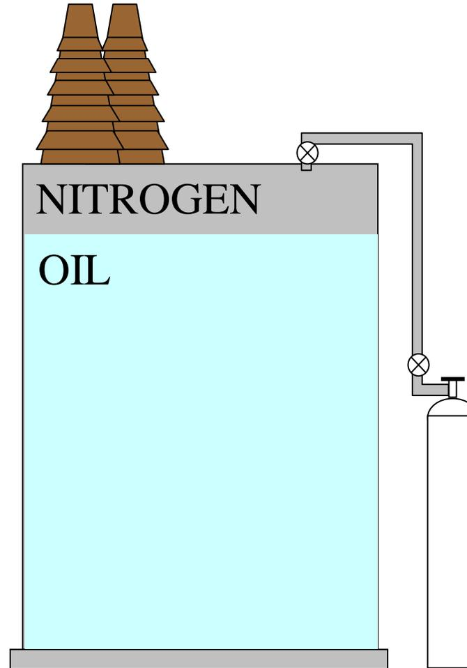
High nitrogen pressure may operate a relief valve during times of high oil expansion due to heating. Nitrogen enters as the oil cools and reduces in volume. There is a low pressure alarm.
