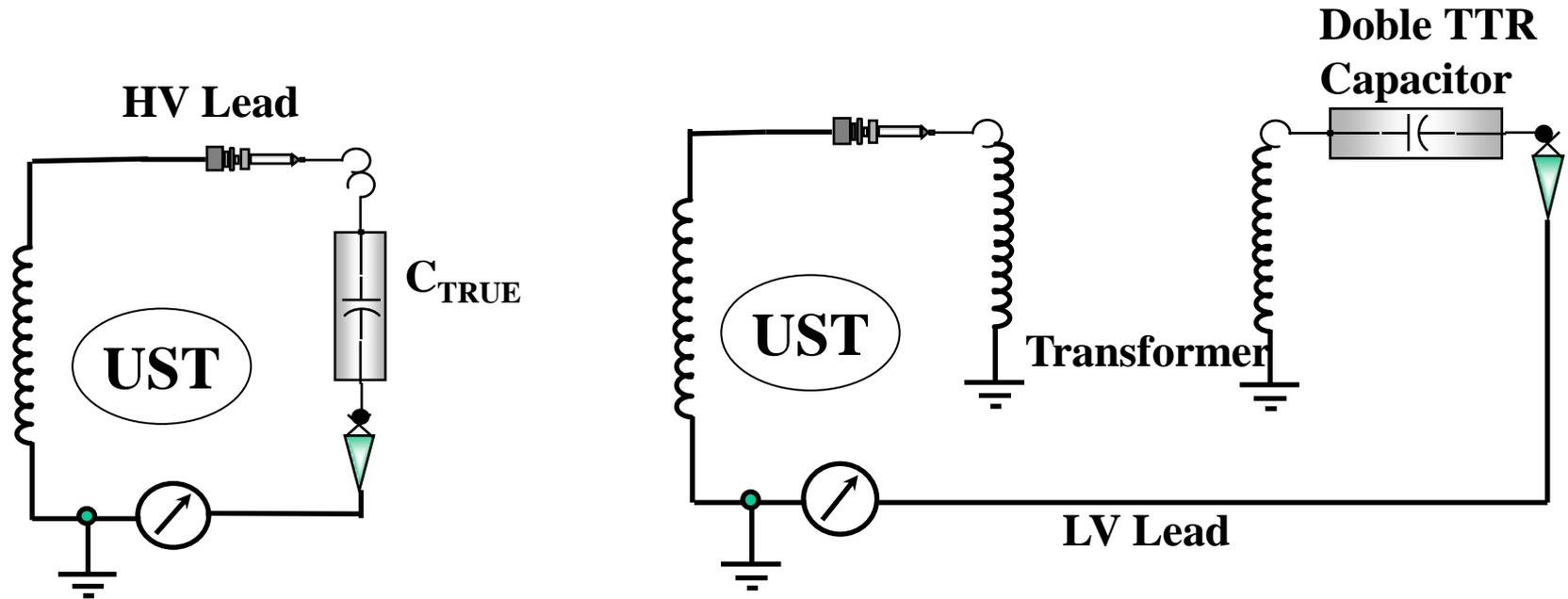
$$C_{True} = \frac{I_C}{10 \text{ kV} \times \omega}$$
