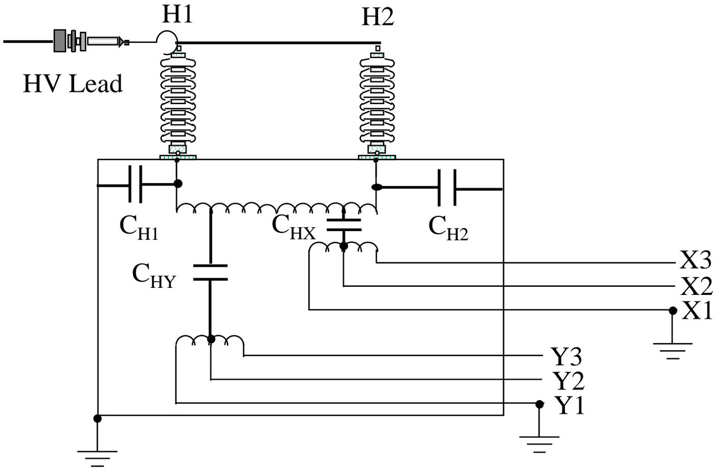
**Test #2 : GST Ground - No LV Lead Required**
