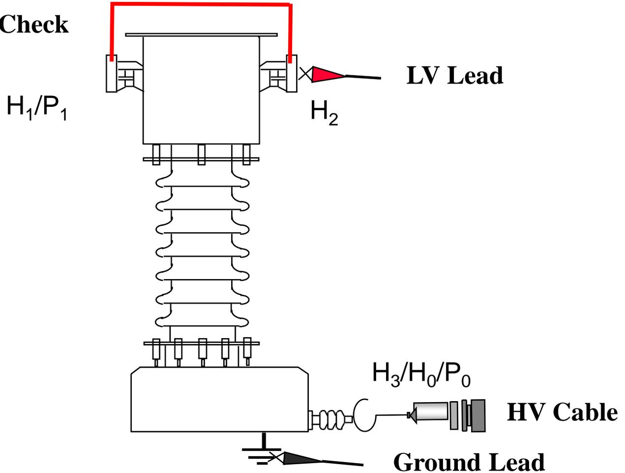
Test kV Limited by Rating of Neutral Bushing (2/5 kV)
