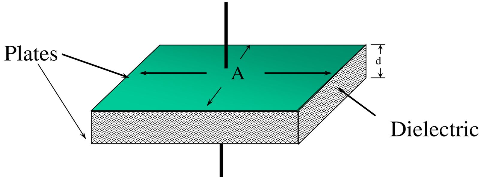
Two conducting plates with area “A” separated by a dielectric with a thickness of “d” and dielectric constant  $\epsilon$
