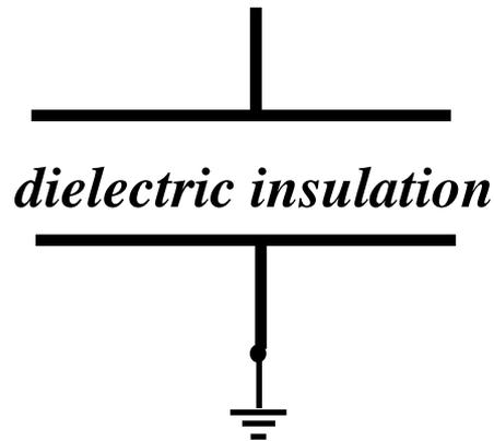
Current generated by polar contaminants in the dielectric shows up as Watts.
