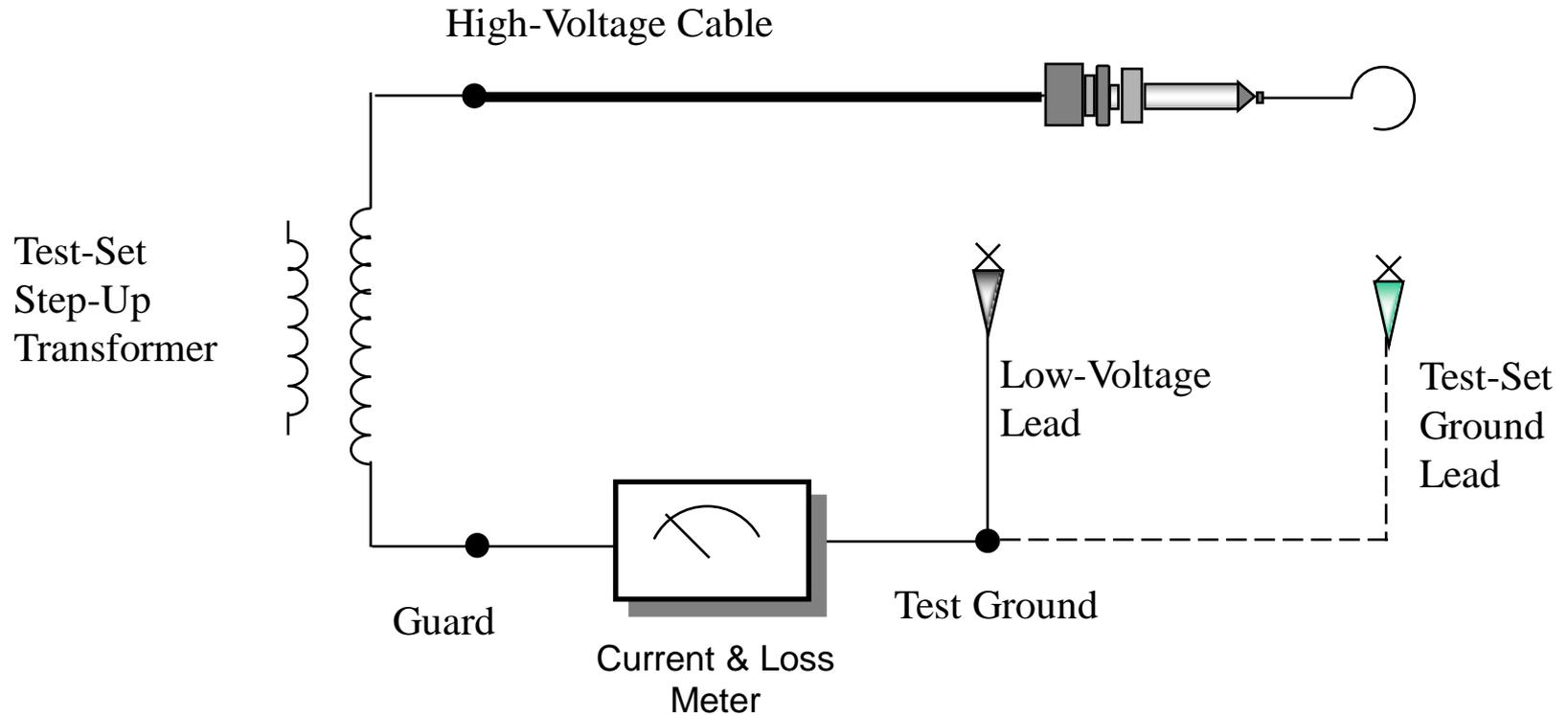
Grounded-Specimen Test Mode (GST-Ground)
