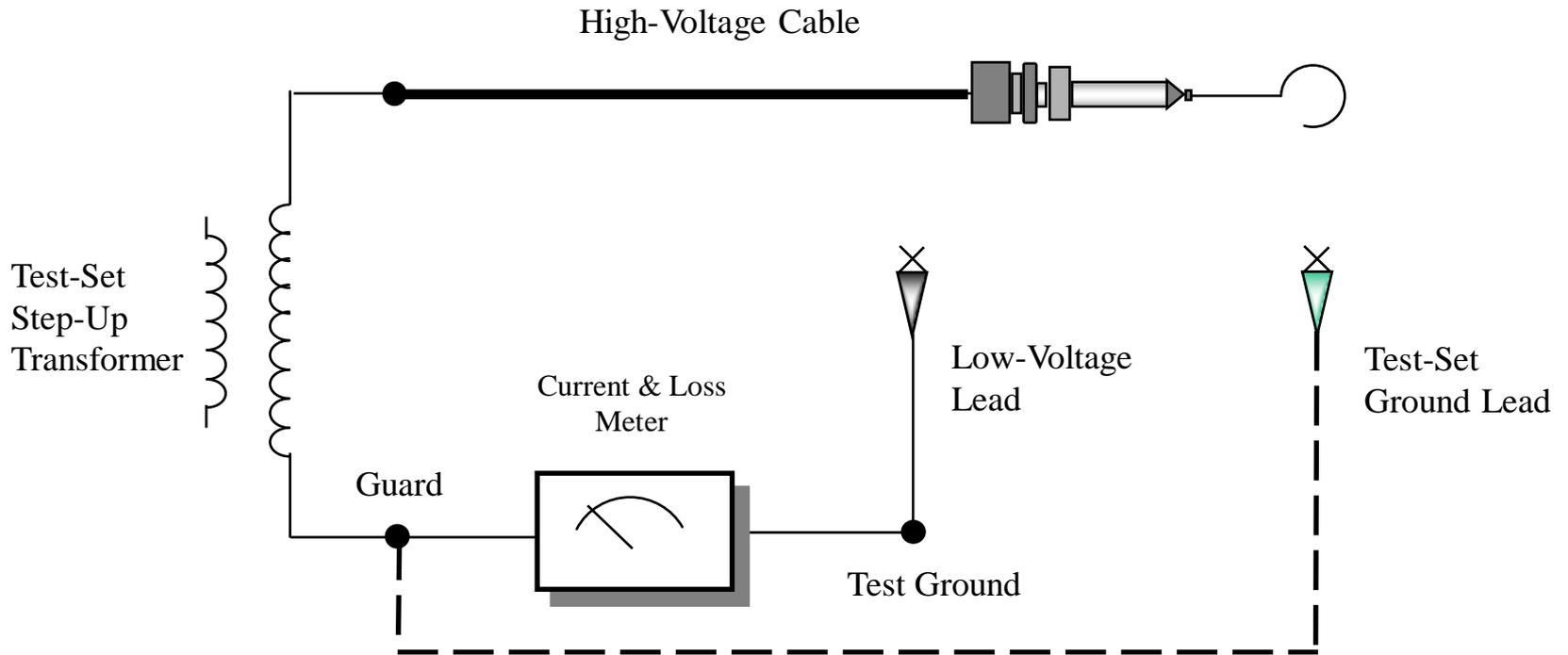
Ungrounded-Specimen Test Mode (UST)
