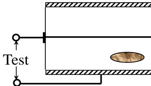
The contamination becomes a “bigger piece” of the insulation and is easier to see
