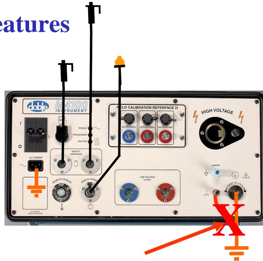
**NEVER** place a jumper from the ground to the “chassis” ground on the test set
