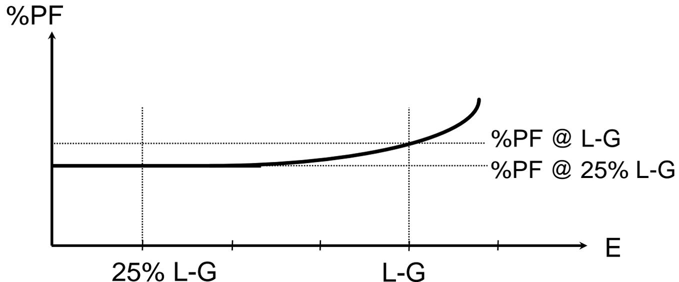
Tip-up occurs in dry-type insulation specimens such as Dry Type Transformer, rotating machinery, and cables.
