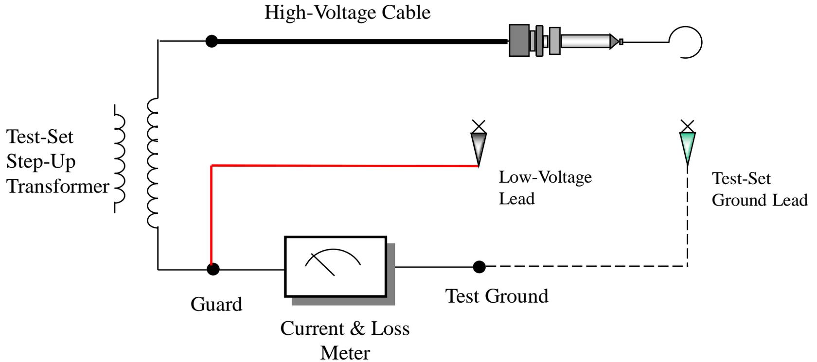
Grounded-Specimen Test Mode (GST-Guard)
