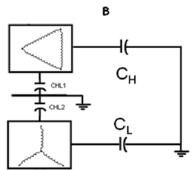
2 winding transformer with grounded electrostatic shield
